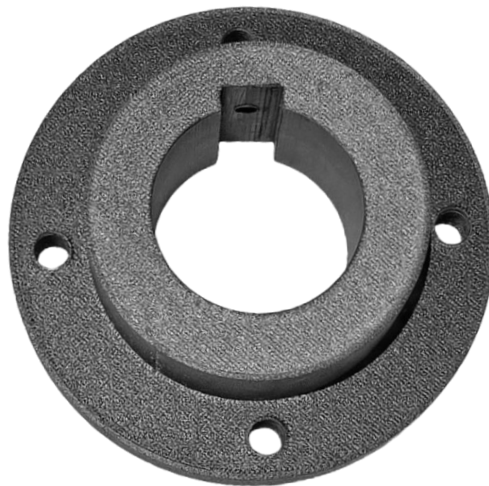
Figure 3: Additively Manufactured Motor Coupling Hub
