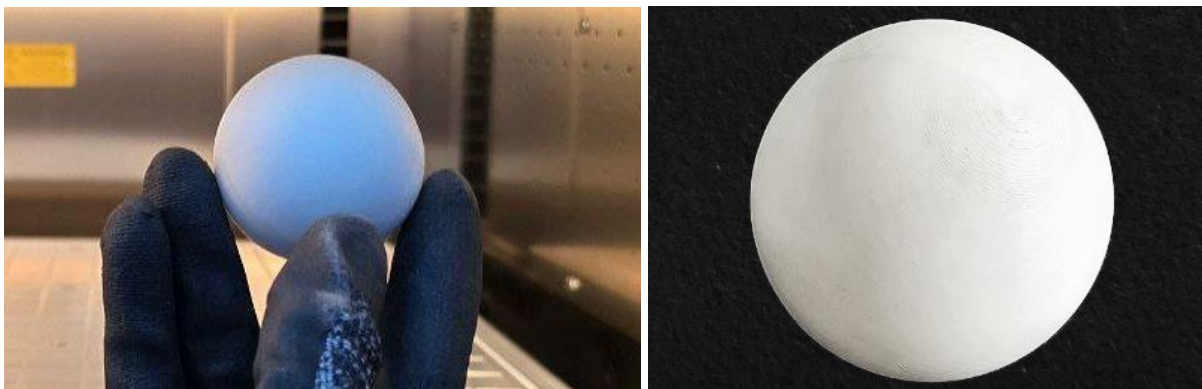
Figure 3: Additively Manufactured Air Release Valve Float
